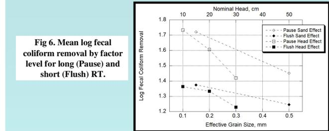
Fig 6. Mean log fecal coliform removal by factor level for long (Pause) and short (Flush) RT.
